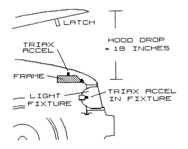
Six channels were recorded, three each from two triaxial accelerometers.  $\,$
