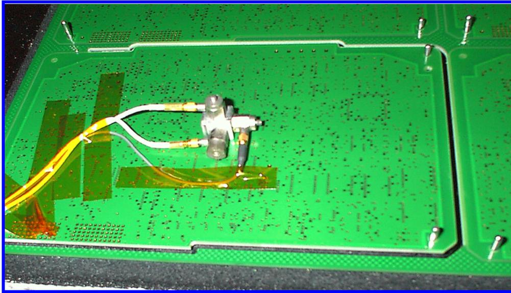
**Figure 1.** Location of triaxial accelerometer array on opposite surface of small board section of larger board panel. Router path can be seen.
